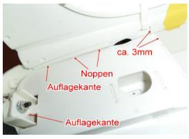
The cabin floor can now be pushed-in from the front of the cab and by pressing a bit the side knobs on the wheel base side covers are locked. You can see below how the tilt limiter should be placed. The floor is then underlaid with the support - everything done.
