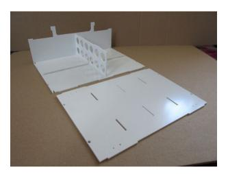
The first end wall can now be attached to the floor. Fronts can be seen the lid lying on the head. The row of grooves in the center is then placed in the assembly in the partition and the end wall.
