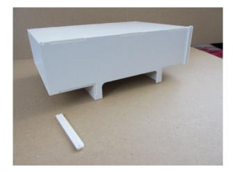
On the box, the bearing strips are adhered now to the four front edges. The hole should come be closer to the forward edge and cover with the slots in the floor.
