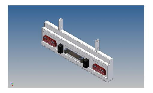
This polystyrene-milled parts set for a bumper as an accessory to the Carson trailer frame (1: 14) designed.
