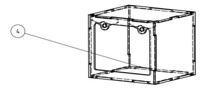
Fit the rear wall (4) back and glue especially all inner edges and the magnetic holder well.
