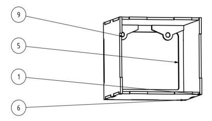
In the two magnet holders (9) each have a magnet (diameter 3 mm - 1 mm thick) is glued so that the magnet surface to the outer side is flush (Magnetic polarity note).
