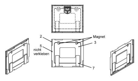
Initially, the lid is assembled, as well as take the frame member (5) as a template to help.
