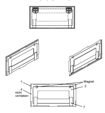
Initially, the lid is assembled, as well as take the frame member (4) as a template to help.
