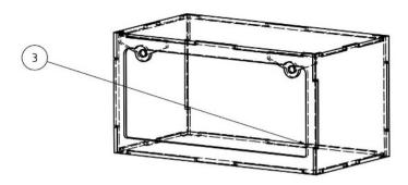
Fit the rear wall (3) back and glue especially all inner edges and the magnetic holder well.
