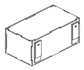
Here in the picture you can see the use of the distance spacers. At its discretion, depending pair a long and short pieces and matching drill holes.
