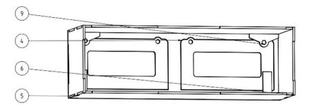
In the two magnet holders (9) each have a magnet (diameter 3 mm - 1 mm thick) is glued so that the magnet surface to the outer side is flush (Magnetic polarity note).
