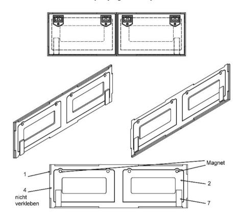
Initially, the lid is assembled, as well as take the frame member (4) as a template to help.
