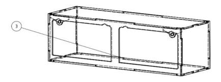
Fit the rear wall (3) back and glue especially all inner edges and the magnetic holder well.
