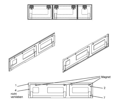
Initially, the lid is assembled, as well as take the frame member (4) as a template to help.
