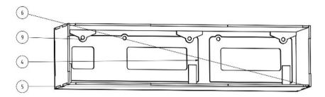
In the two magnet holders (9) each have a magnet (diameter 3 mm - 1 mm thick) is glued so that the magnet surface to the outer side is flush (Magnetic polarity note).
