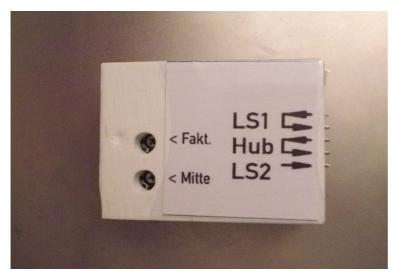
On the left you can find the potentiometers for setting the gain (Fakt) and the center (Mitte) of the second steering servo.
