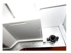
You can clearly see how the cab floor is pushed from the front to the rear support and how the tilt limiter should be placed.
