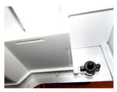
You can clearly see how the cab floor is pushed from the front to the rear support and how the tilt limiter should be placed.
