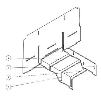
Fitting the support parts (4) to (6).
