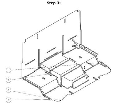
Mount the floor parts (8) (left and right) and the front cap floor (9) on the slots provided or respectively on the form elements, align and glue them together.
