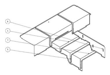
Fitting the support parts (4) to (6).
