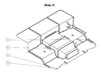
Mount the floor parts (8) (left and right) and the front cap floor (9) on the slots provided or respectively on the form elements, align and glue them together.
