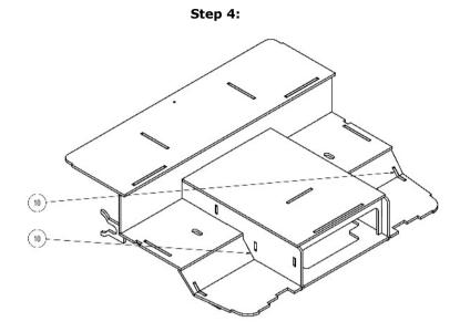
Mount the footwell parts (10) (left and right) between the side parts (2) and the joining aids (11) and (12) respectively.
