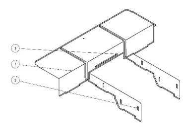
Glue the side parts (2) to the cab bed plate (1) right-angled and flush fitting. The slots in part (1) would be helpful for this action
